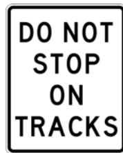
Figure 7-6. DO NOT STOP ON TRACKS Sign.
